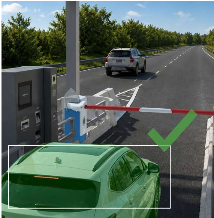
Vehicle type recognition enabling automatic application of the appropriate pricing rules
